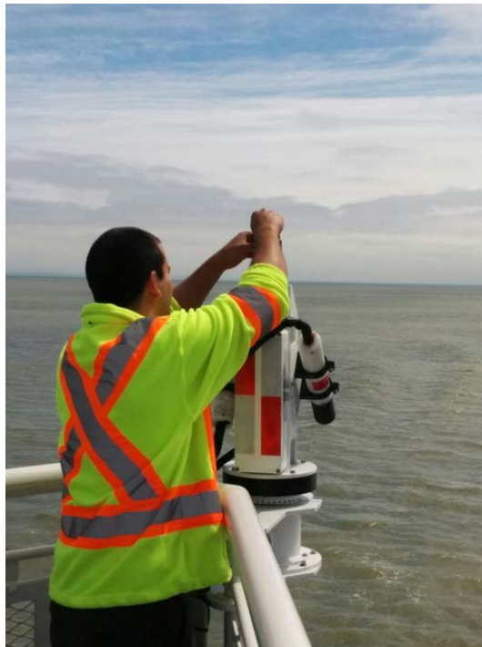
SAS Solar Tracker - cleaning
